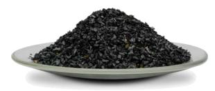
Crushed Tungsten Carbide material is fully sintered tungsten carbide hardmetal that has been crushed and pulverized with sizes from 200 mesh to 1/4 inch.
