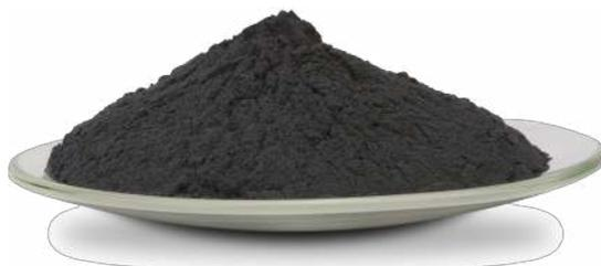
High Purity Tungsten Powders produced at Buffalo Tungsten are typically greater than 99.999% in tungsten content. Impurity analyses are performed by EAG labs using GDMS method for accurate low level results.
