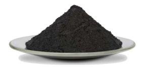
The WS Series is a second grade tungsten powder specifically for non-sintering applications where the high density of tungsten is desired yet extreme purity is not required. WST powder has a larger particle size with higher tap and apparent densities.
