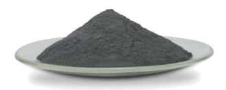
Our Coarse Tungsten Powders are typically greater than 99.9% purity with average particle sizes from 10 to 50 microns. They have higher apparent density and better flow properties than Fine Tungsten Powder.
