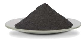
Co-Reduced Tungsten Powder is made by the addition of metal powders to the tungsten oxide prior to the reduction process, resulting in higher green strength after compaction. Common additives are nickel, copper and iron in any amounts. These powders provide excellent wear properties while remaining machinable.
